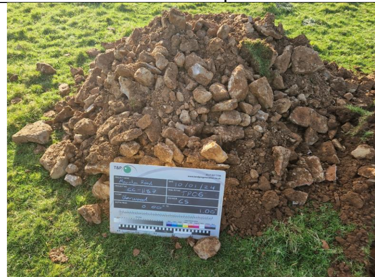
PLATE 12 – Trial Pit Spoil – TP06.
