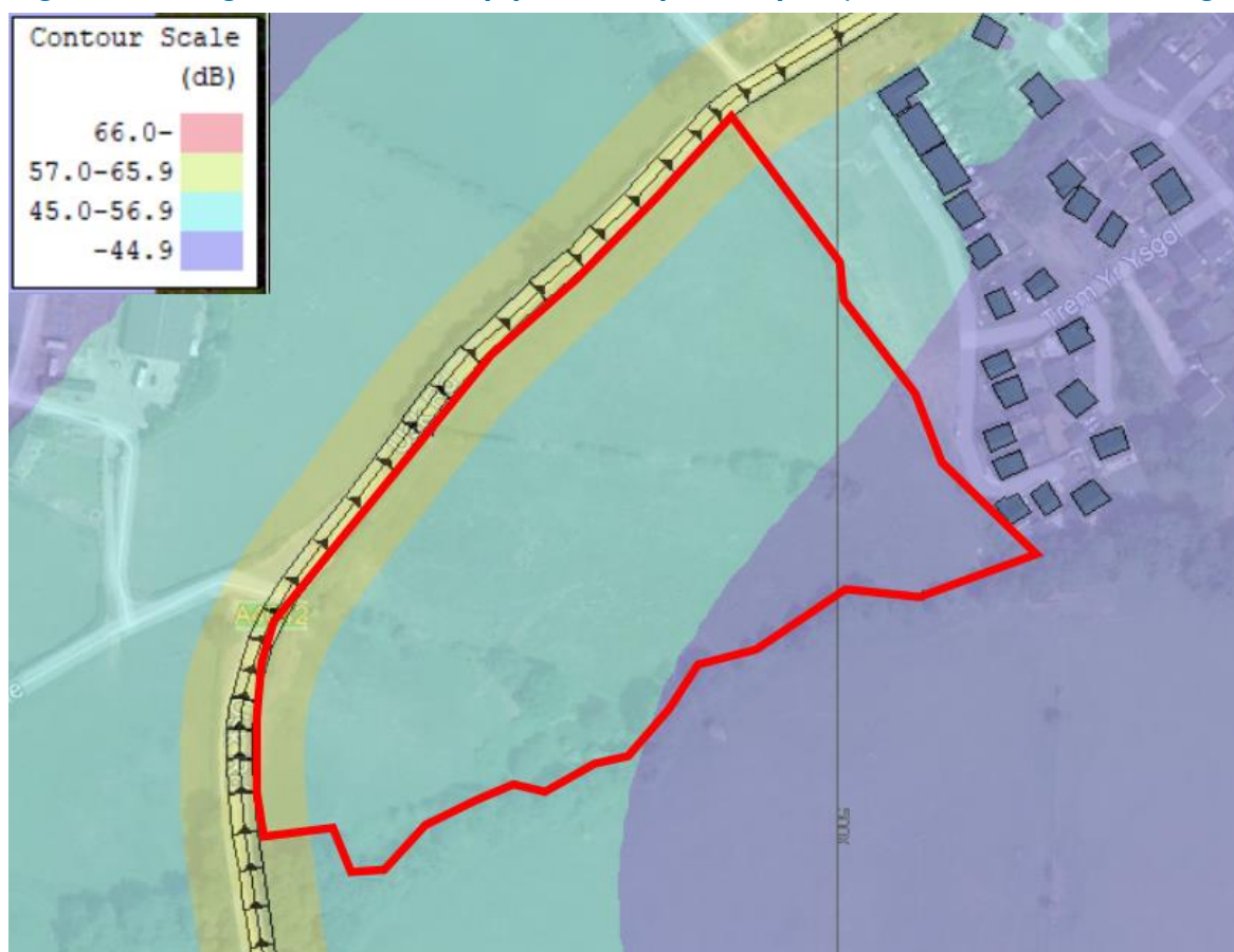
Figure B.9 – Night-time Noise Map (Undeveloped Site) L_{Aeq,8hr} Contours at 1.5m Height
