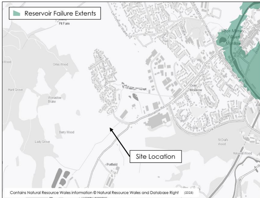
Figure 3.3: NRW Reservoir Failure Extents
