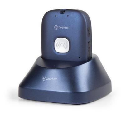
GPS mobile social device (neck work) – can be set to call registered contact numbers for family to either alert when the wearer exits the property (linked to the base via Bluetooth, when Bluetooth is disconnected it raises the alert) or a safe zone can be set. Safe zones would be set via geofence area on a map which allows the wearer to go out in a zone and if they go out of this area then the alert is triggered, can also be set to alert when the person comes back into the safe area.
