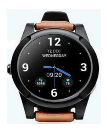
GPS mobile social device (wrist worn) — can be set to call registered contact numbers for family to either alert when the wearer exits the property (linked to the base via Bluetooth, when Bluetooth is disconnected it raises the alert) or a safe zone can be set. Safe zones would be set via geofence area on a map which allows the wearer to go out in a zone and if they go out of this area then the alert is triggered, can also be set to alert when the person comes back into the safe area.
