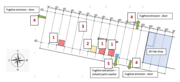
**1** – Item identifies the Graco spray pumps that are attached to the 1000L IBC. Generally this is a closed system with no escape of VOC to atmosphere.
