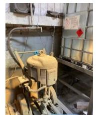
Paint is applied by airless spray via a pressurised air line and paint Graco paint gun.
