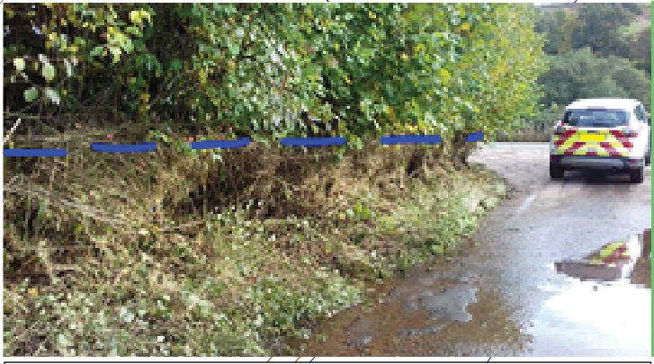
Debris accumulations along hedge (height indicated by blue lines)
