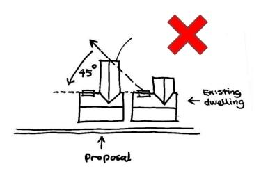
7.13 Developments which do not meet these standards (the 25° rule and 45° splayline) will normally be resisted unless it can be demonstrated by the applicant that it
