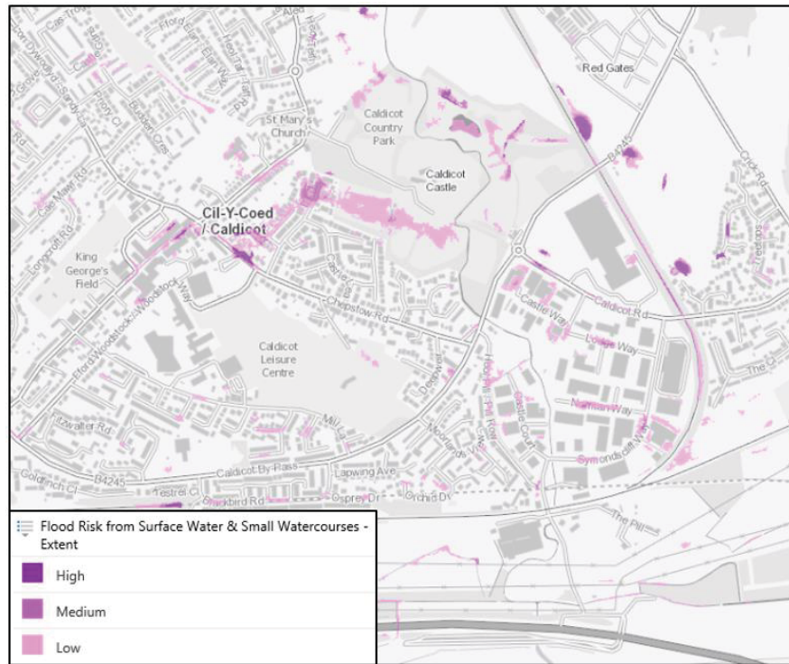
Figure 7: Extract from Natural Resources Wales Flood Map showing the Risk of Flooding from Surface Water
