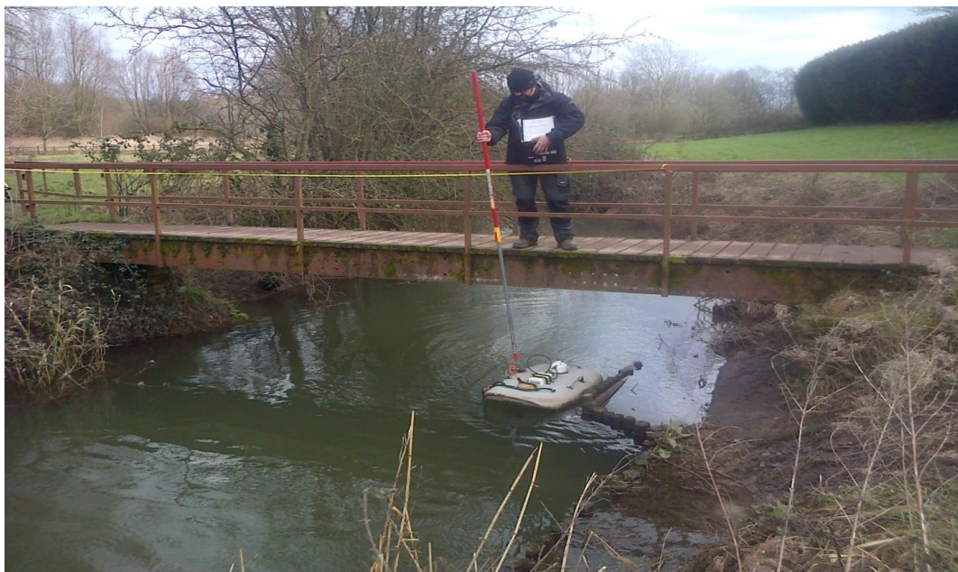
Figure 1 Flow gauging at ‘Nedern DS’ using a Sontek M9 ADCP view south (Photograph with permission of Hydrometry & Telemetry Team South East Wales, Natural Resources Wales)
