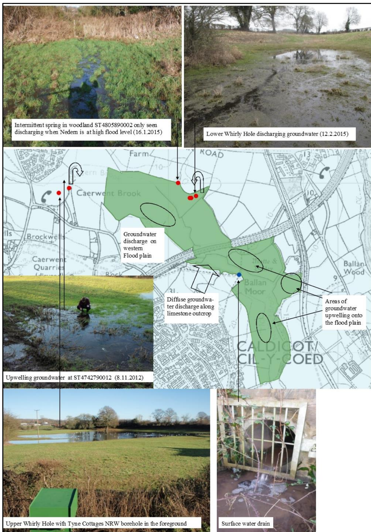
Figure 5 Key groundwater and surface water discharges in the Nedern SSSI (P502171, P915237, P915234, P915243). © BGS NERC.
