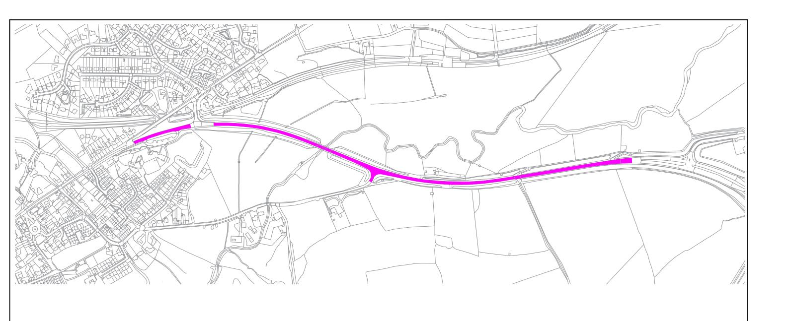
A472 Usk, Completion Date 13/09/2018, 14mm CGSC, 60 PSV, 1160 Tonnes, Inlay, 40mm Thick
