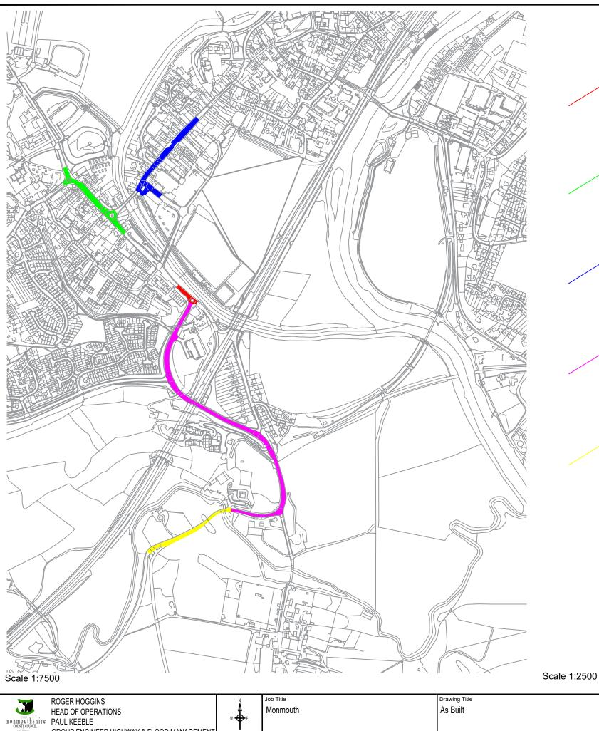
Cinderhill, Completion Date 10/10/2018, 10mm CGSC, 65 PSV, 160 Tonne, Inlay, 40mm Thick
